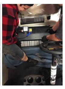
9. Lower the battery pack all the way into the battery tray in the golf car. After the battery pack is fully in and seated in the golf cars battery tray, remove the blanket.
