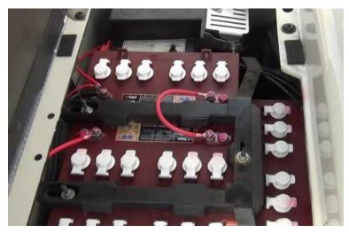
3. Remove the red power cable running from the battery pack to the contactor. Cut away the attached yellow wire to the power cable. This wire will need to be fitted with a 5/16" ring connector. Discard the original red battery cable.
