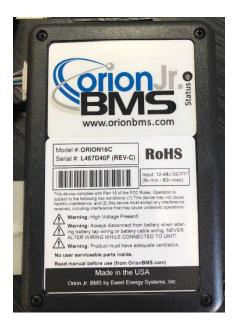
1. With the power cord plugged in to the delta-q charger, the OrionJr. BMS will be powered as well. If the BMS is functional without any errors, the status indicator light will illuminate green. (Fig. 37)
