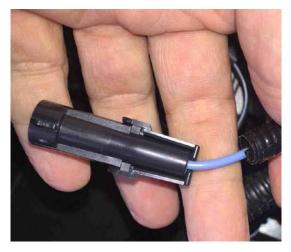
HPEVS supplied connector in wiring harness
