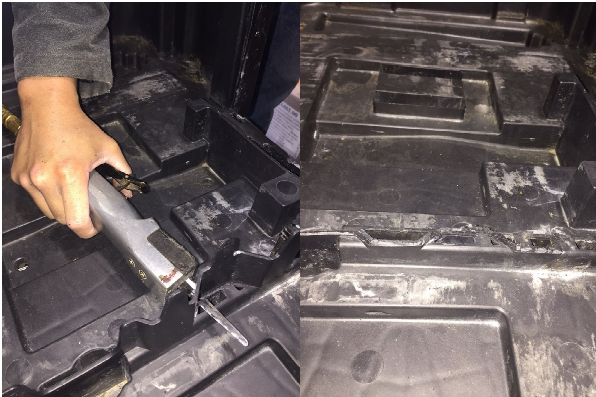
Fig. 6- Raised material removed.
