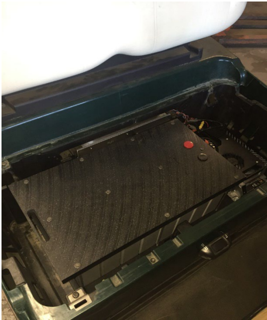
Fig. 18-Lithium battery pack installed into golf car
