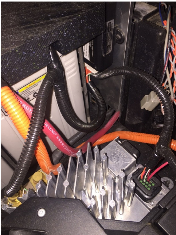
Fig. 1- Cable routing from battery pack
