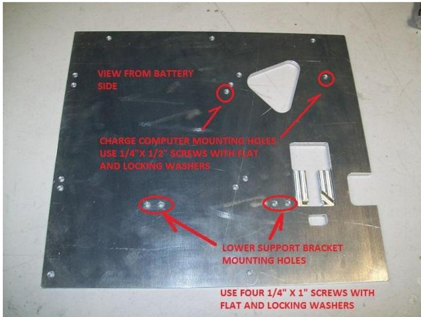
2. Install the lower support brackets. See above picture for hole locations. Use four  $\frac{1}{4}$  x 1" screws, flat and lock washers. Make sure that the screws do not protrude to the other side of the plate. The lower support bracket should create a "hook" or gap where the controller plate will be mounted in the car. See pictures.
