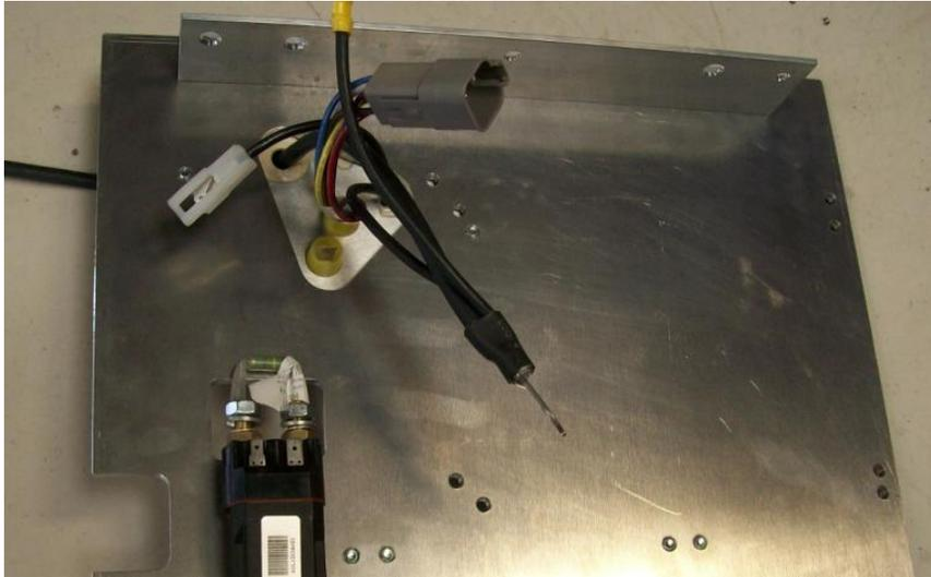
5. Install the AC controller. Similar to the stock controller, the controller is mounted on the motor side of the car. Depending on the controller used in a particular application, different sized screws will be used. For 1238 and 1236 controllers use four  $\frac{1}{4}$  x  $1\frac{1}{4}$ " screws, and lock washers. For 1234 controller, use four  $\frac{1}{4}$  x  $\frac{1}{2}$ " screws, and lock washers. The following picture shows the location of the mounting holes.
