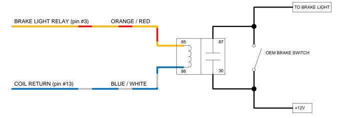
\*\* This option turns the brake lights ON during REGEN. Brake TYPE 5 allows for NEUTRAL BRAKING AND/OR BOOSTED REGEN while pressing the brake pedal. Brake TYPE 2 & 3 uses a variable input for BOOSTED REGEN.
