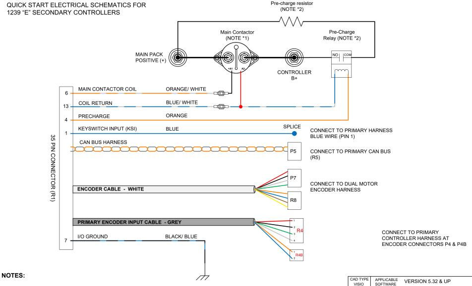
(\*1) Use supplied contactor. (GIGAVAC Part #GV200PA-1). Use only a Contactor WITHOUT PWM AND COIL SUPPRESSION. FAILURE TO DO SO CAN CAUSE CONTROLLER FAILURE AND WILL VOID WARRANTY.
