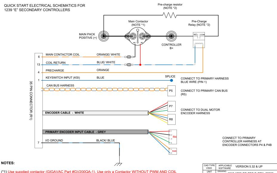
(\*1) Use supplied contactor (GIGAVAC Part #GV200QA-1). Use only a Contactor WITHOUT PWM AND COIL SUPPRESSION. FAILURE TO DO SO CAN CAUSE CONTROLLER FAILURE AND WILL VOID WARRANTY.
