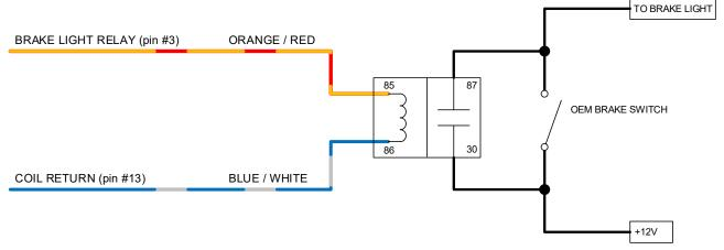
\*\* This option turns the brake lights ON during REGEN. Brake TYPE 3 allows for NEUTRAL BRAKING AND/OR BOOSTED REGEN while pressing the brake pedal. Brake TYPE 1 & 2 uses a variable input for BOOSTED REGEN. Brake TYPE 0 does not allow for BOOSTED BRAKE while pressing the brake pedal.
