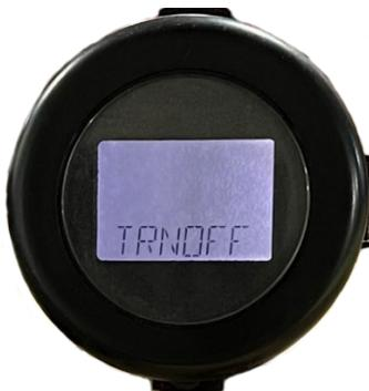
9. The motor controller is now programmed with the throttle inputs. Cycle the key switch and drive the car to verify the throttle functionality.
