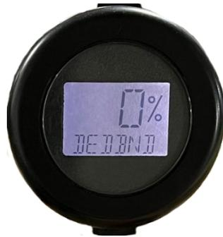
7. Slowly depress the throttle foot pedal until the display shows that the dead band has been set. The 3140 display will show the following when the dead band has been set. The numerical value will or will not be the same as shown.
