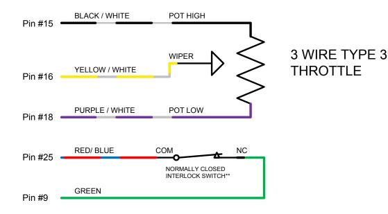
\*\* When the accelerator pedal<u>IS PRESSED</u> the interlock switch is released to its <u>NORMAL</u> position (switch not activated) thus completing the circuit since its green wire is connected to the normally closed (NC) connection.
