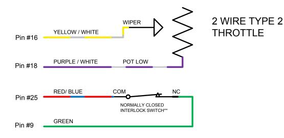
\*\* When the accelerator pedal <u>IS PRESSED</u> the interlock switch is released to its <u>NORMAL</u> position (switch not activated) thus completing the circuit since its green wire is connected to the normally closed (NC) connection.
