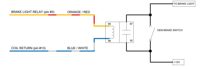
\*\* This option turns the brake lights ON during REGEN. Brake TYPE 0 does not allow for BOOSTED BRAKE while pressing the brake pedal. Brake TYPE 1 & 2 uses a variable input for BOOSTED REGEN.
