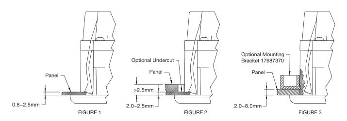
**NOTE:** Mounting bracket 17687370 can be used for panel thicknesses 2.0–8.0mm. Mounting bracket is designed for one installation only. Destruction of mounting bracket may occur if attempted to remove.
