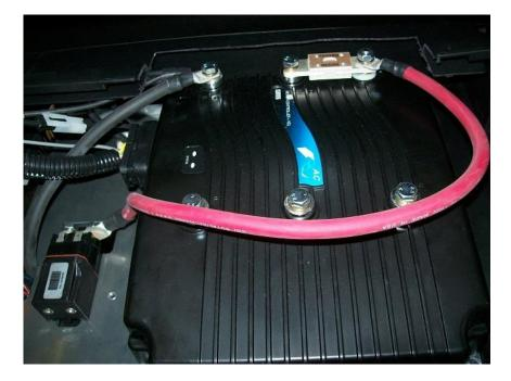
9. Install the red 20 cable from contactor's Hot side to the (+) positive side of the pack. Make sure that the terminal lug does not touch the plate. As an added precaution a cable boot may be used.
