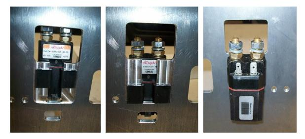
4. Install the upper mounting plate bracket. The upper mounting bracket is facing the motor side of the car. Use three 1/4 x 1/2" screws, flat and lock washers. There is no need to fully tighten the screws at this step. The bracket's wider side will be mounted on top of the car similar to the stock controller bracket.
