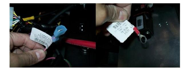
13. Re-connect the stock contactor coil wires (Light blue and Blue/ white).
