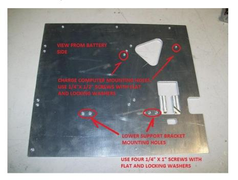
2. Install the lower support brackets. See above picture for hole locations. Use four ¼ x 1" screws, flat and lock washers. Make sure that the screws do not protrude to the other side of the plate. The lower support bracket should create a "hook" or gap where the controller plate will be mounted in the car. See pictures.
