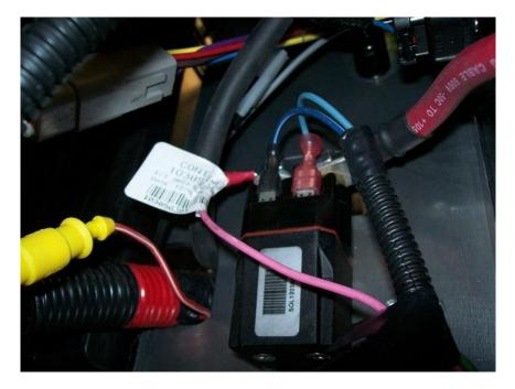
14. Locate the 6 pin grey connector from the stock harness. Locate and cut the brown/ white wire. Install a male ¼" quick disconnect and connect to the brown wire from the new system harness.
