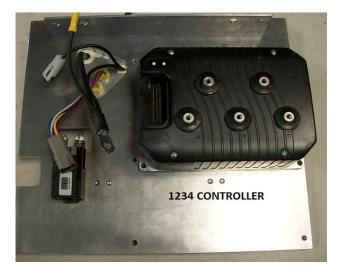
6. Install the AC controller plate in the car. The lower support bracket should insert the battery pack tray. The upper bracket should rest on top of the battery pack tray. Reuse the black screw saved from the removal of the stock controller. Use the supplied two ¼ x ¾" self tapping screws. Once these three screws are secured, proceed to tighten the upper bracket to the plate screws that were loosely installed earlier. See pictures.
