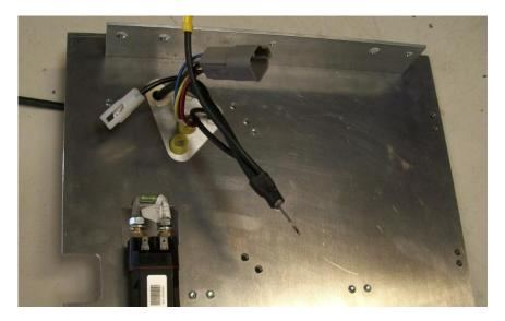
5. Install the AC controller. Similar to the stock controller, the controller is mounted on the motor side of the car. Depending on the controller used in a particular application, different sized screws will be used. For 1238 and 1236 controllers use four ¼" x 1¼" screws, and lock washers. For 1234 controller, use four ¼ x ½" screws, and lock washers. The following picture shows the location of the mounting holes.
