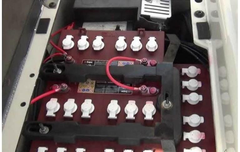
3. Remove the red power cable running from the battery pack to the contactor. Cut away the attached yellow wire to the power cable. This wire will need to be fitted with a 5/16" ring connector. Discard the original red battery cable.
