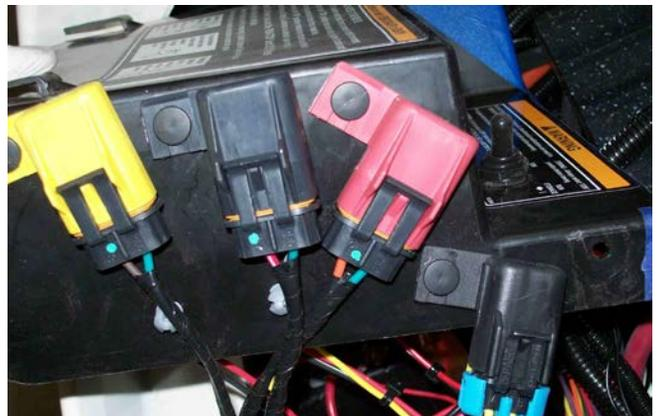
3. After relocating the fuse holder, note the blue area on the controller splash guard depicted in the picture (Fig.9). This material needs to be cut away.
