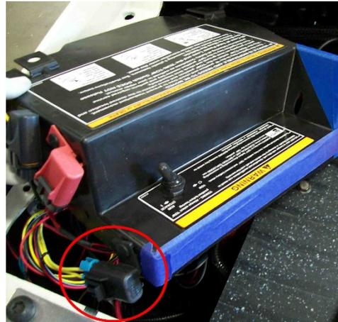
2. Relocate the fuse holder to the next hole to the left of the original placement. The location is seen in the picture and is circled in yellow. (Fig.8)
