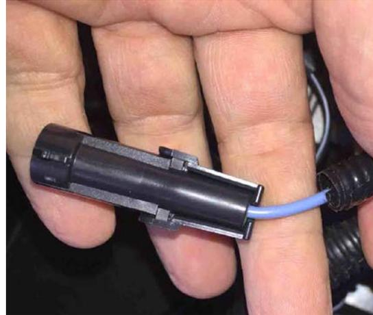
HPEVS supplied connector in wiring harness
