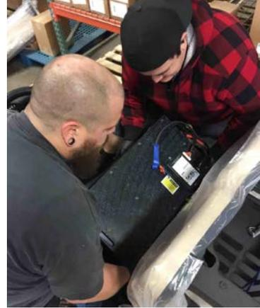
8. Make sure that the standoff studs that are located on the bottom of the battery pack clear the lip of the body.
