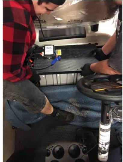
9. Lower the battery pack all the way into the battery tray in the golf car. After the battery pack is fully in and seated in the golf cars battery tray, remove the blanket.
