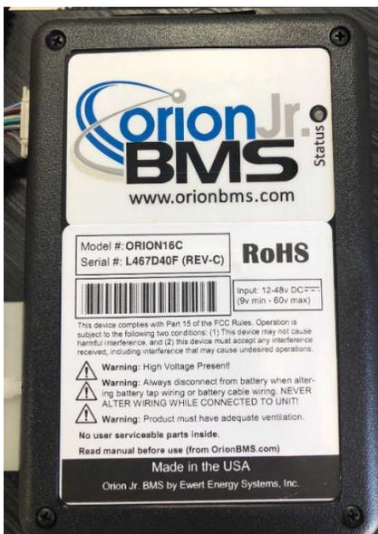
1. With the power cord plugged in to the delta-q charger, the Orion Jr. BMS will be powered as well. If the BMS is functional without any errors, the status indicator light will illuminate green. (Fig. 37)
