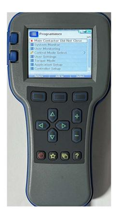
The installed Curtis 3140 display will also display current faults. When a fault is active, the display will show the letter "C" followed by the two digit fault code; i.e., for a main contactor did not close fault, the fault code will be C39. If there are multiple faults, the faults will display in succession.
